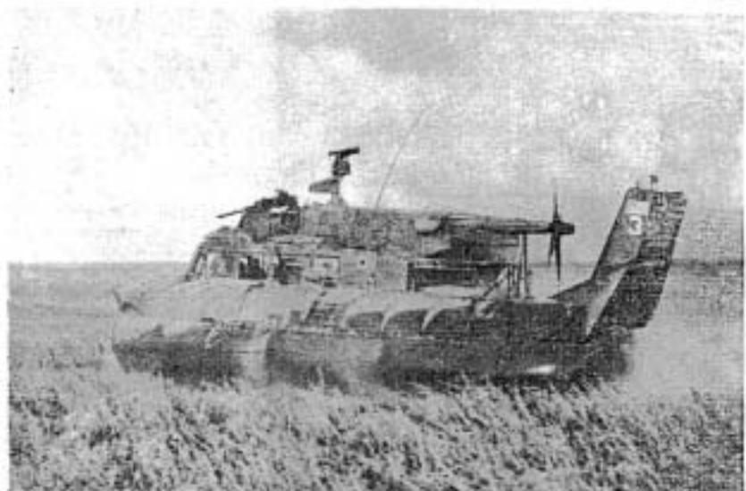
IT'S A BOAT? IT'S A PLANE? . . . Actually it's some of both. It has no draft, because it is supported by a cushion of air created by a fan inside its body and forward propulsion is caused by a propeller.
